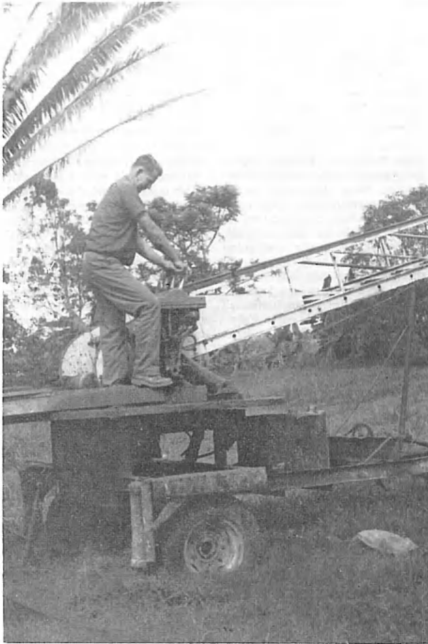
Mennonites in Spanish Outlook recycle junk to produce useful machines. Menno Loewen, an M.D.S organizer in the Kleine Gemeinde Community displays his hydraulic crane constructed from a ladder truck.
