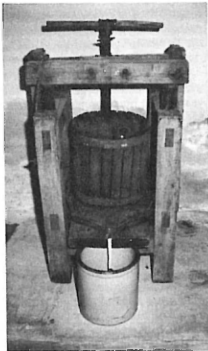
A wine press built by Jacob H. Goering, Pretty Prairie, Kan., about 1885. It was used to press juice from grapes, apples, and other fruits grown by the pioneers. (Owned by Walter W. Graber, who will donate it to the Mennonite Centennial Village, Bethel College.)
