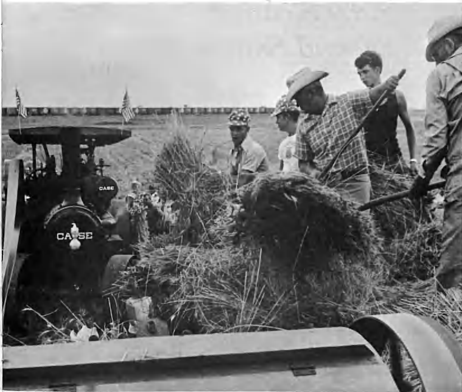
During the Newton, Kan. centennial observance in July 1971, residents of the area had an opportunity to see a demonstration of how wheat was threshed in by-gone days. Bundles are pitched into the threshing machine (foreground), powered by a massive steam tractor with long belt drive.
