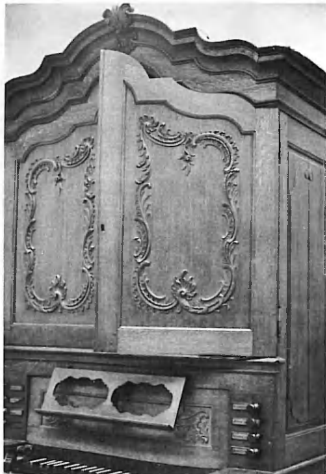
The Flemish Baroque case of the organ is oak. The design on the door is carved out of the panel, not glued on. The organ has seven stops for five and a half ranks of pipes. Some stops draw only the upper or lower half of the keyboard. Keys are of ebony with ivory sharps, just the opposite of modern keyboards.
