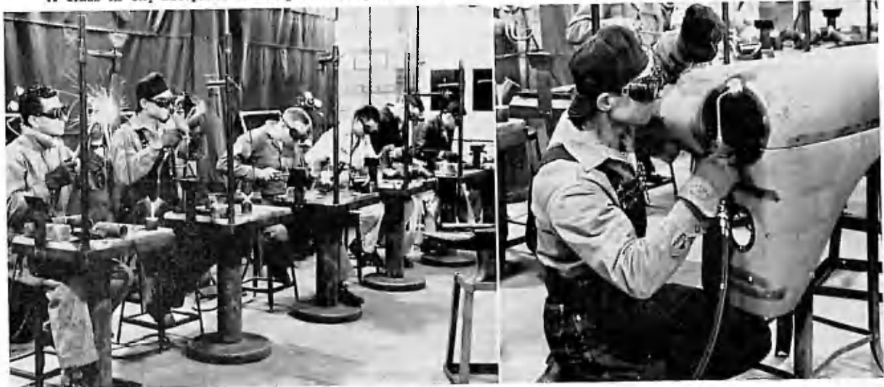
A class in oxy-acetylene welding and body-lender repair, a useful application of oxy-acetylene welding.
