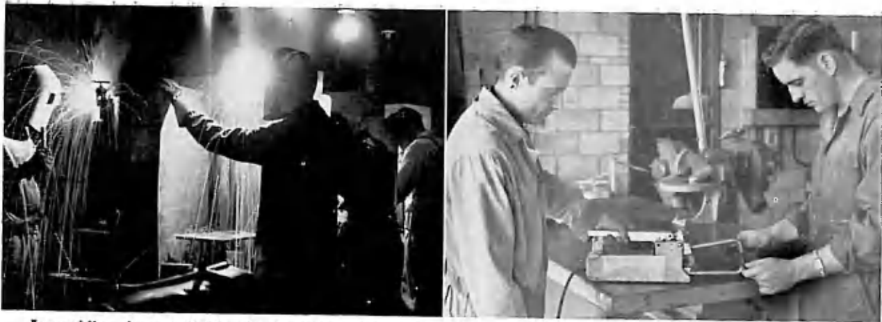
Arc-welding, largest division in the department, and resistance welding, used primarily with light sheet metal.
