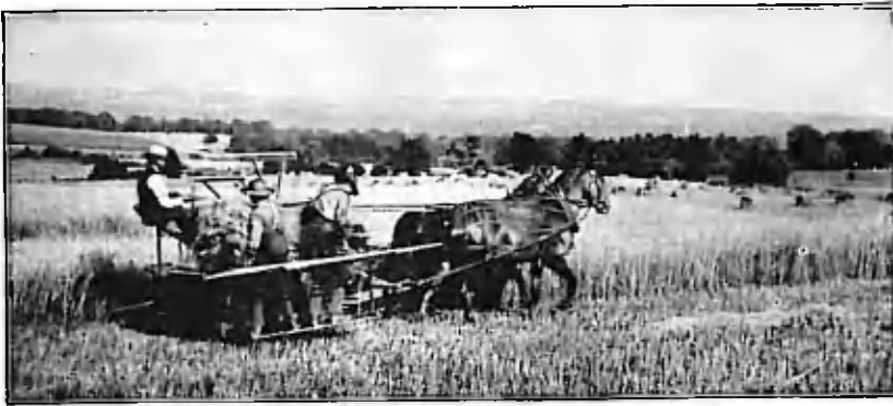
Here we see the binders riding on the reaper. Thus two men did the binding which formerly needed 4-5 men.
