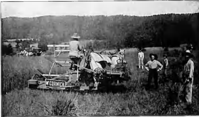
The first self-binder attracted spectators from far and near. Wire was used to tie the bundles.
