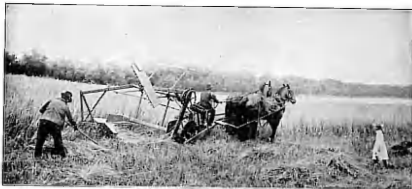
The next step was the self-rake reaper known as the "Old Reliable," a one-man machine built in 1864.
