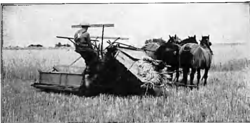
This binder, made since 1888, had a bundle carrier and other improvements. Harvesting was now a joy.
