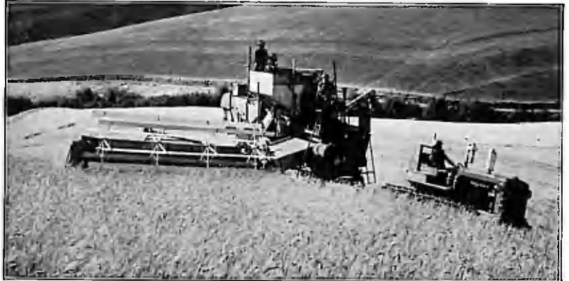
A fourteen-foot combine pulled by a Caterpillar tractor makes large harvesting crews unnecessary.
