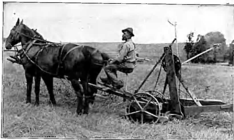
The "Advance," a reaping and mowing machine produced 1869-1879. The platform could be removed for mowing hay.
