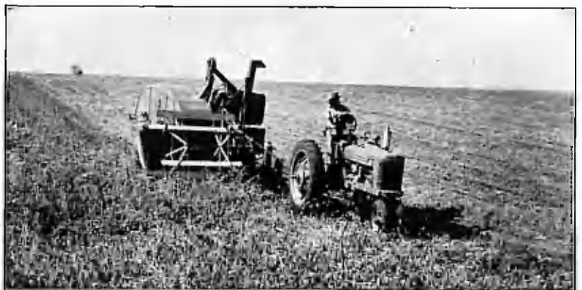
This six-foot combine is an all-purpose harvester for the average farmer. Here it is used to cut and thresh soybeans.
