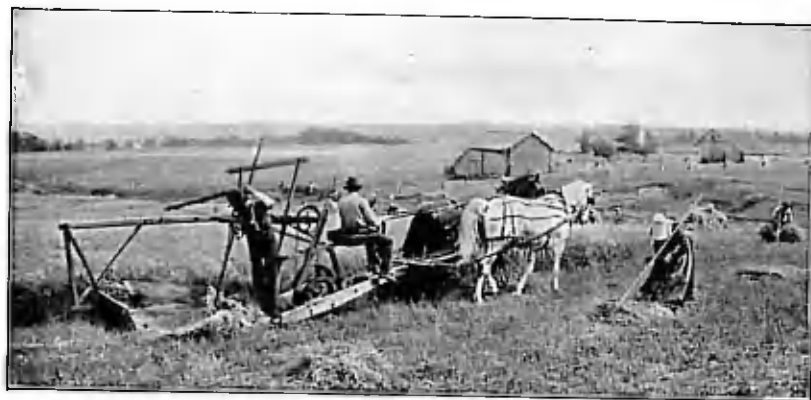
An advanced reaping and mowing machine built in 1857. Note addition of seat for driver.
