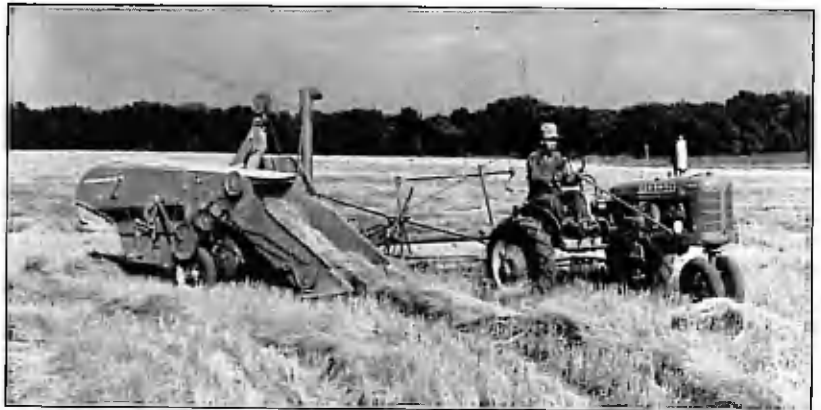
The six-foot combine used on many farms threshes standing grain or grain previously cut and laid in windrows.
